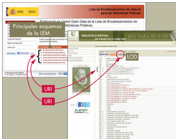
Diagram showing the FHL Virtual Libraries link with the LEM through MARC21 fields which are transformed dynamically in RDF records linked through their URI.
